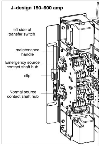
Figure 1-6. Maintenance handle on 150–600 amp. J–design transfer switches. Hubs shown with Normal contacts closed & Emergency open.
